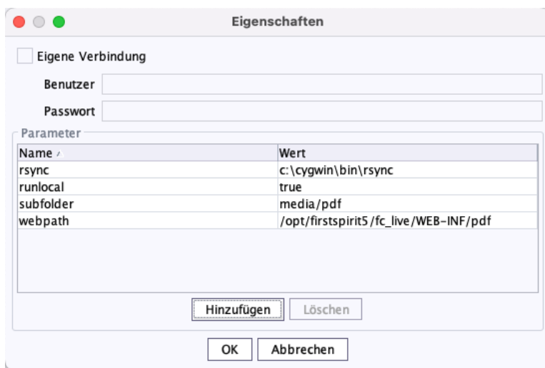
Figure 4.40. Sample configuration for the PDF action deployment script on a Windows server
